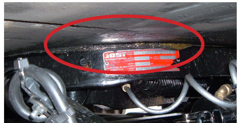
No gaps between fifth wheel and upper coupler
